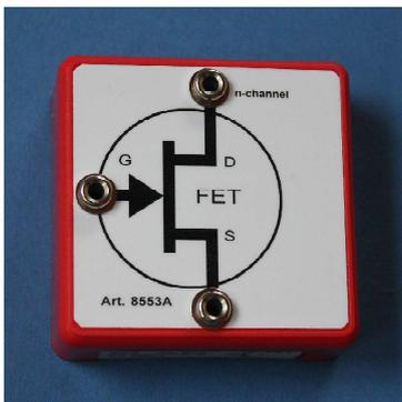
**Junction-Feldeffekt-Transistor Typ J133, n-Kanal**
