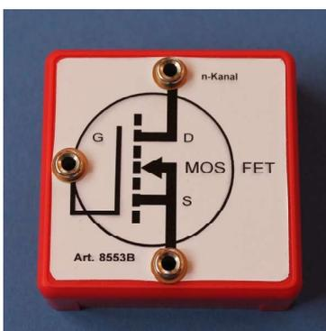
**MOSFET, n-Kanal, 100 V, 5.6 A, TYP IRF510PBF**
